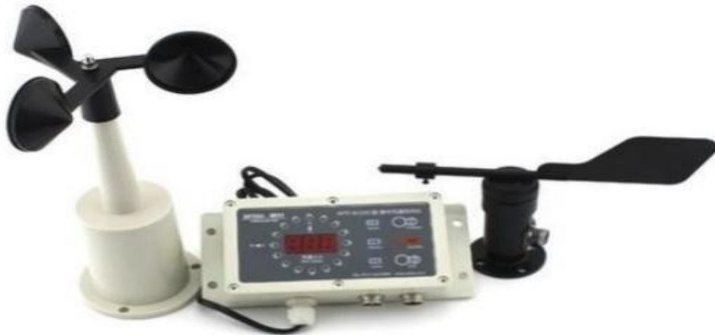
Figure 11 Wind measurement system
