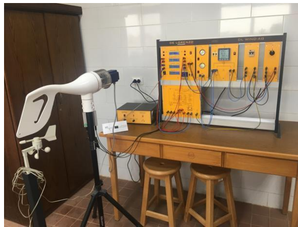
Figure 9 Lab2 Wind Energy setup integrated with measuring instrument
