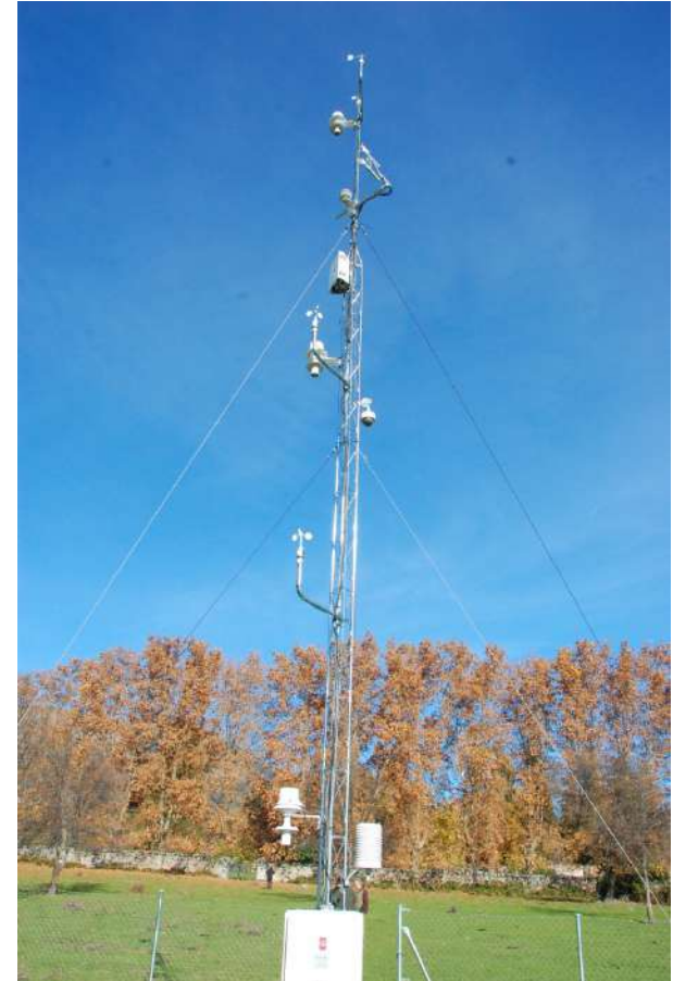
Anemometric tower. Source: Universidad Complutense Madrid
