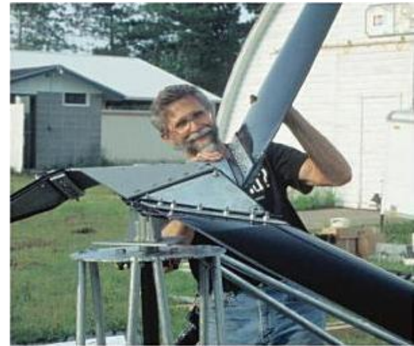
Polypropylene blades with flexible hinge on a downwind turbine.
